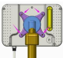
On the back of the product, 4 M4 75\*75mm thread holes are reserved, and the hole position of the bracket (refer to the left) is aligned with the thread hole, and the screw is screwed into the M4 specification.
