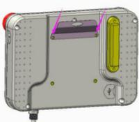
Through sketch left hanging structure, specifications of the screws fixed in the shell reserved above two holes, can suspended in a desired position control.
